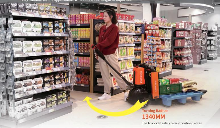
The frame of the PTE15Q truck is surrounded by steel covers making the truck looking different and also ensuring the protection of components.
